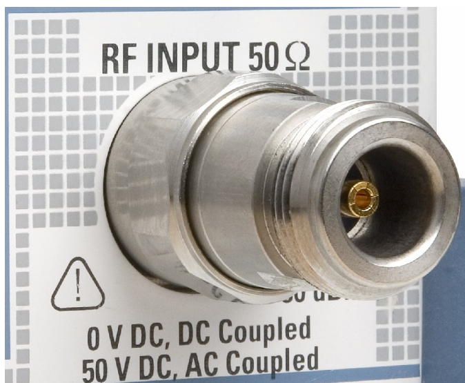
Figure 3: Attached Test Port Adapter Head (N female)
