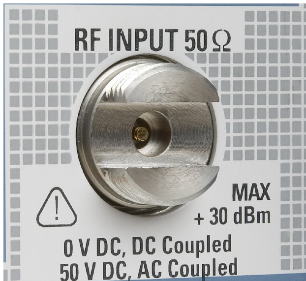
Figure 1: Test Port Adapter Body
